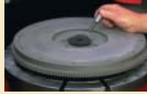
3. Install the centering cone, hold down the bolt, and tighten
