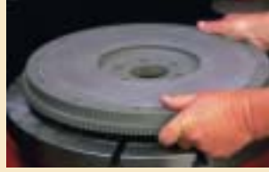
2. Lay the flywheel on the adapter
